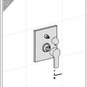
Fix the control valve body on the valve box (please confirm the orings on the bottom of control valve is not missing).
