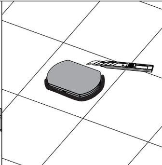
5. Cut the extra plaster shield, seal the gap with waterproof sealant.
