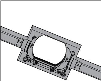
4. Fixing the box by cement and get the tiles cutted according to the cover dimension.
