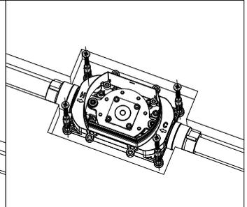
3. Use the screw driver to fix the valve to the floor by the screws provided.
